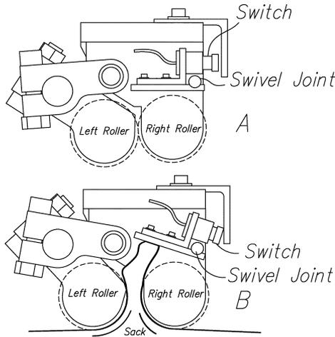
Fig. 8. Switch issues a signal when enough sack material is collected between the rollers.
