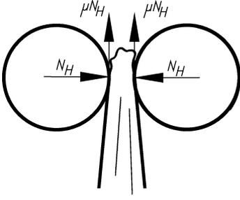
Fig. 14. Friction forces prevent the sack from sliding out.
