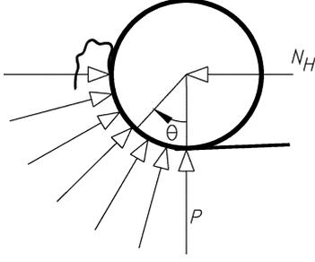
Fig. 13. Pressure profile on the end-effector roller.
