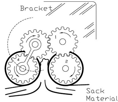
Fig. 4. When the rollers come in contact with a sack, the gears turn the rollers inwardly to grab and drag the sack into the end-effector via frictional forces.
