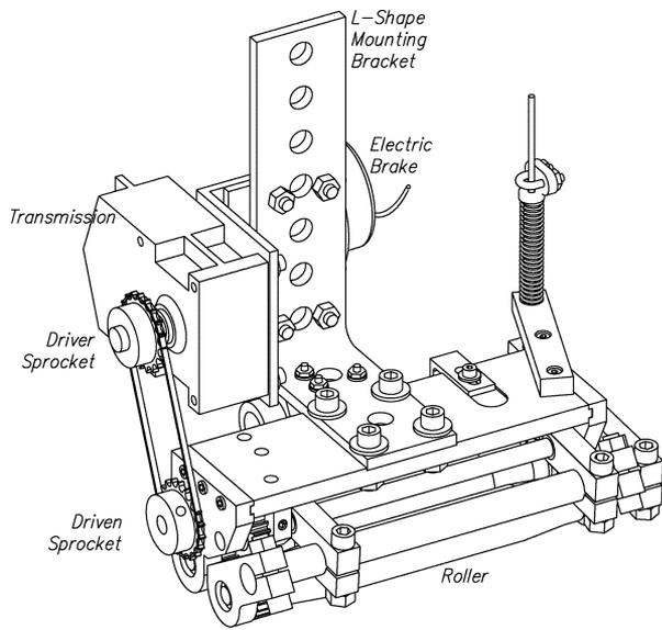
Fig. 5. Driver sprocket is secured to the transmission output shaft of the speed reducer transmission. The driven sprocket turns a shaft, which powers the grasp mechanism underneath the horizontal plate.
