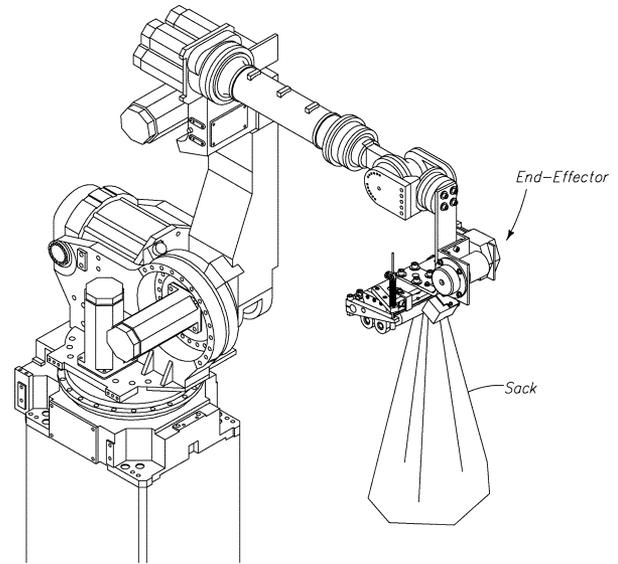
Fig. 9. Fanuc robot and the end-effector holding a sack.
