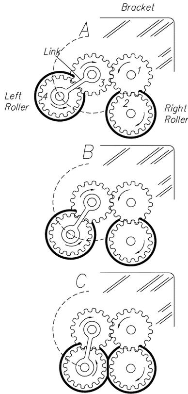
Fig. 3. Link shown above is not connected to Gear 3 and turns independently of Gear 3. The rotation of the link along the dashed line allows the rollers to come in contact with each other or separate from each other.
