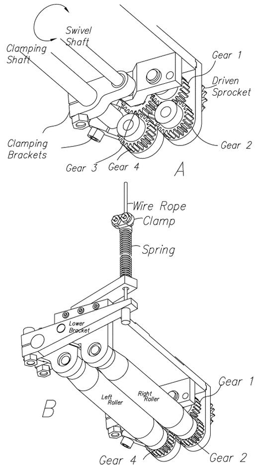
Fig. 7. (a). Beneath the end-effector with the rollers removed. (b) Spring that pushes the left roller against the right roller.
