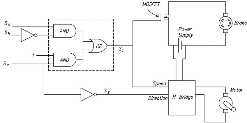
Fig. 11. Schematic representation of how  $S_G$ ,  $S_H$ , and  $S_R$ , drive the events and operational phases of the end-effector.
