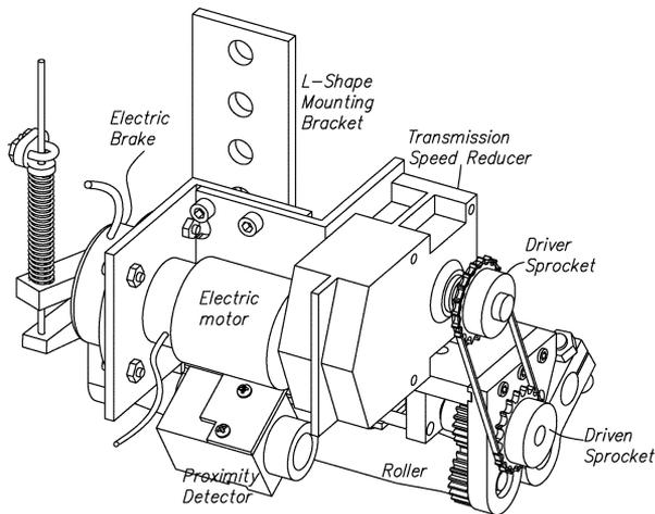
Fig. 6. Electric brake is installed on the mounting bracket to lock the motor when needed. When the brake is not powered electrically, it is engaged, preventing the motor shaft from turning.
