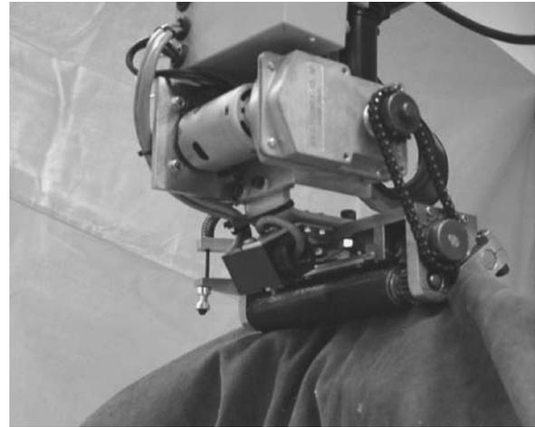
Fig. 15. Robot and the end-effector holding a sack.
